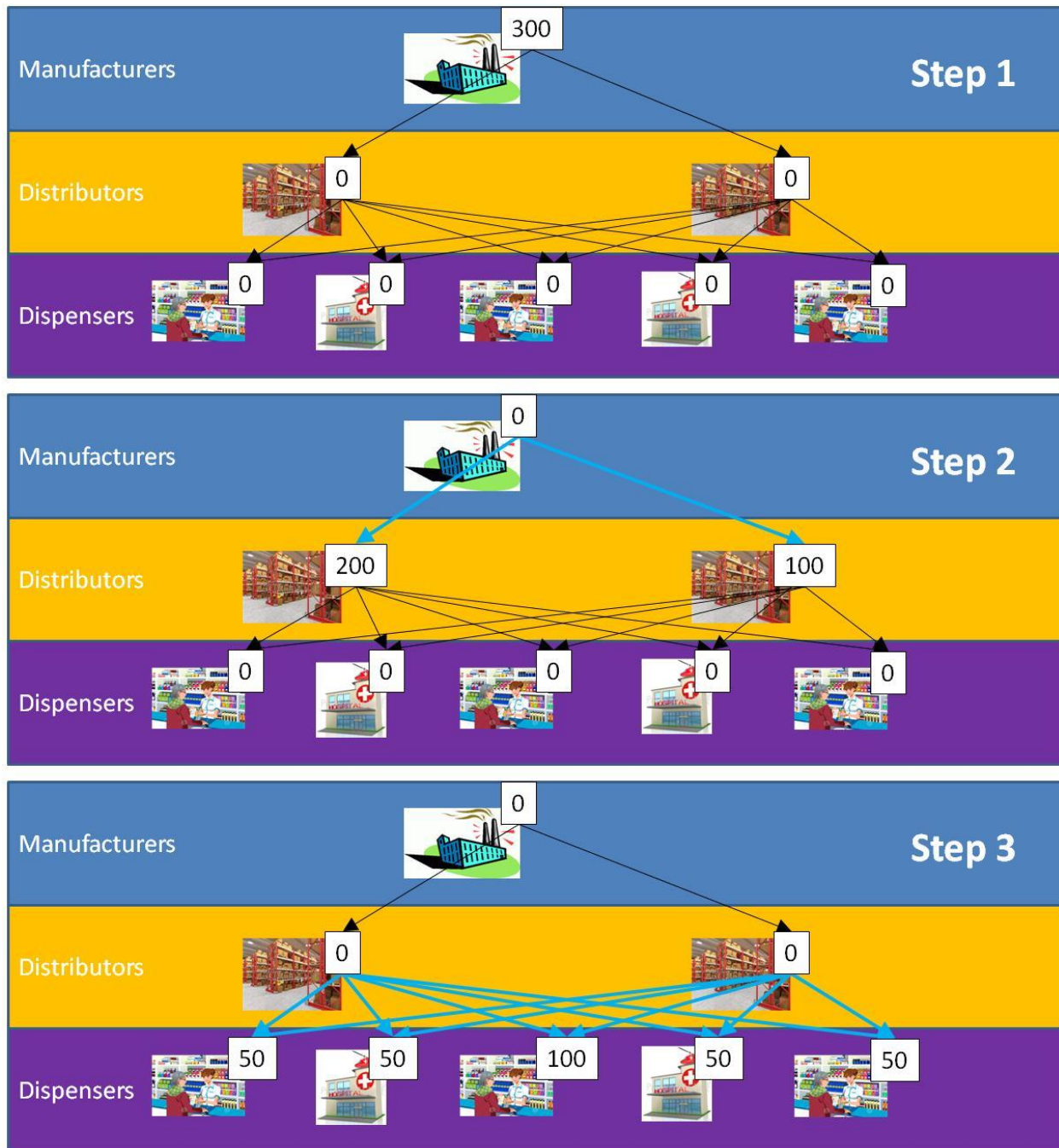
Figure 1: Change of Ownership Tracking. By tracking the input and output flows from each member of the supply chain, "the system" is able to maintain visibility of the path of dissemination of a particular product to recognize which parties have how much inventory. But individual supply-chain members can only see their immediate upstream and downstream transactions.
